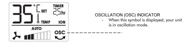
5. **SET THE SLEEP TIMER (TIMER):** The timer function allows you to set the length of operation of your heater from 0.5 hour to 7.5 hours. Pressing the **'Timer'** button repeatedly will increase the length of operation by 0.5 hour each time. The sleep timer can be set in any mode.
