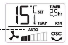
3. **SET THE TEMPERATURE YOU WANT (UP** and **DOWN)**: When the unit is in the AUTO MODE ONLY, the LCD will display a '**SET TEMP**' (Set Temperature) indicator. The digital temperature readout display will be flashing (see figure).
